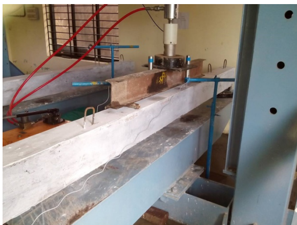
Fig. 8. Loading and deflection measuring set up
