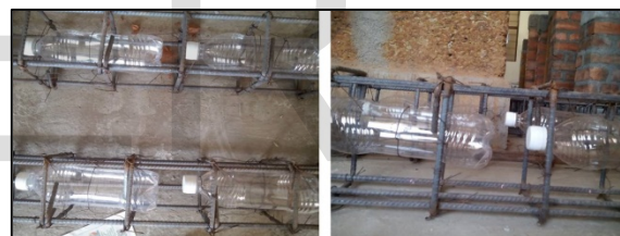
Fig. 7. Reinforcement cages for voided beam with spacing
