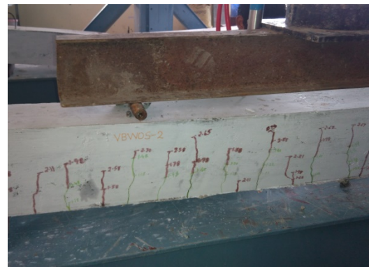
Fig. 13. Crack formed in VBWOS-2
