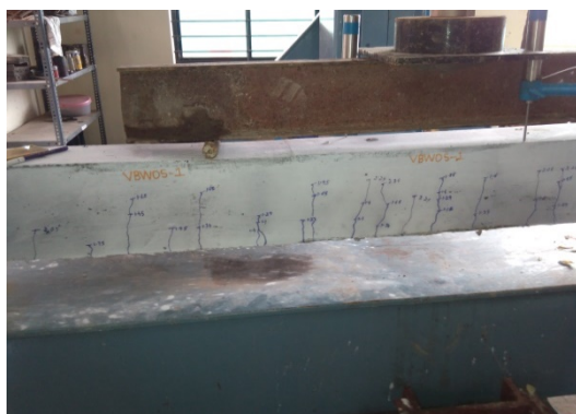
Fig. 12. Crack formed in VBWOS-1
